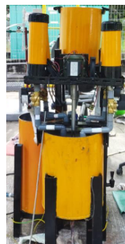
Figure 5. Automatic Machine for Converting Waste Cooking Oil into Aromatherapy Candles
